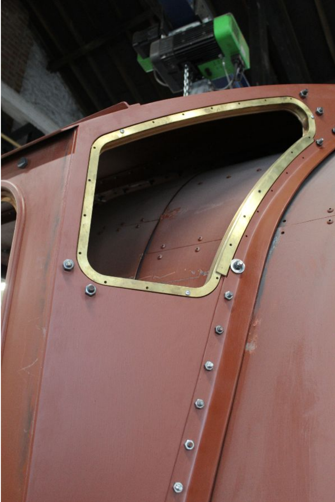
Trial fit of right-hand cab spectacle window frame - David Elliott/A1LST
