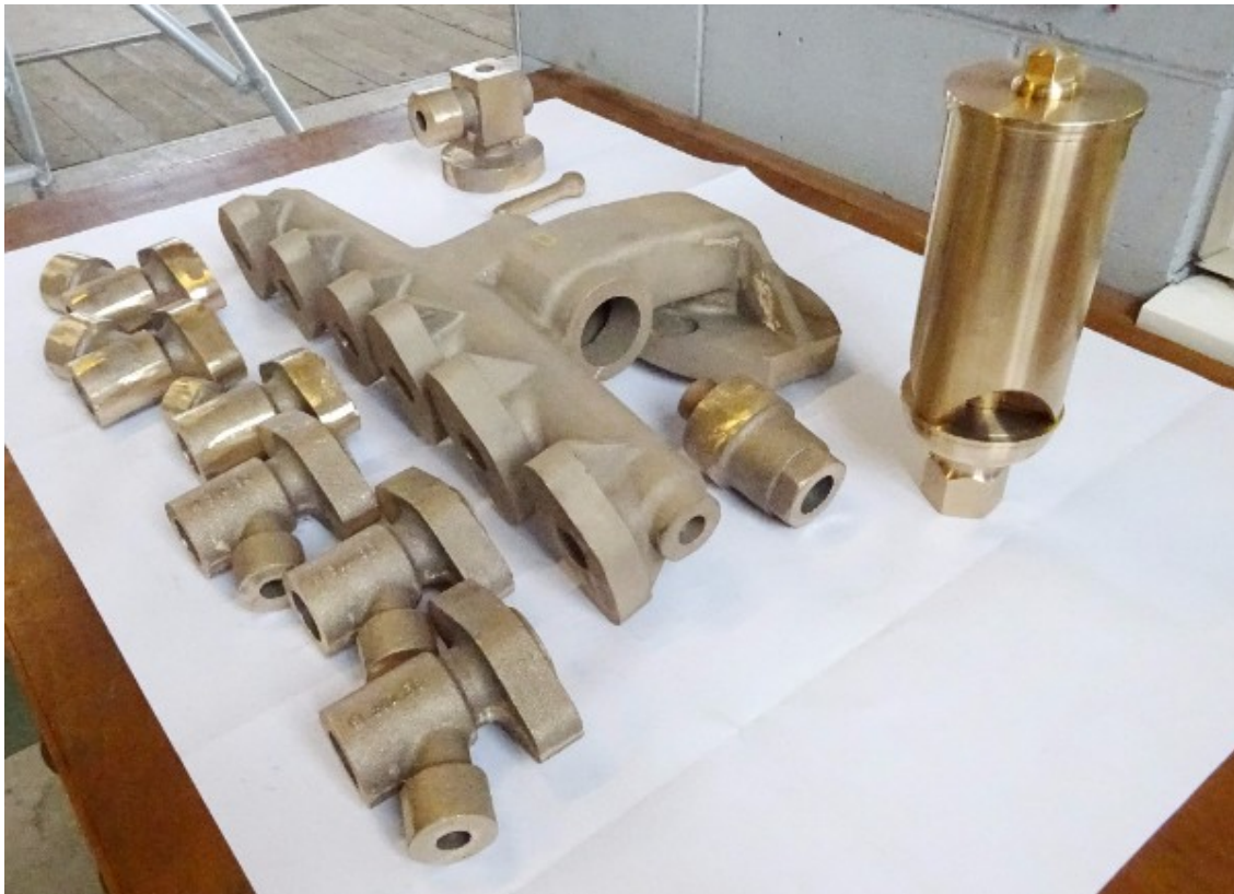
Boiler manifold and components and the chime whistle – David Elliott
