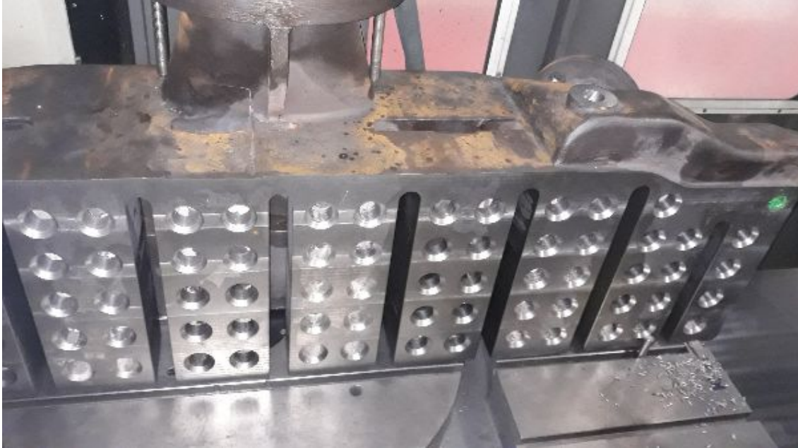
Superheater header being machined - David Elliott/A1SLT
