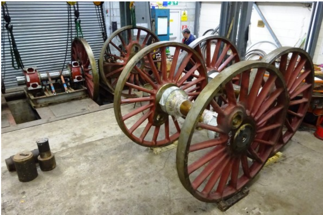
With two driving axles complete, a third is assembled at SDR(E) - David Elliott
