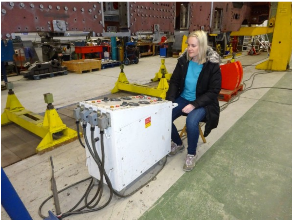
Daniela Filova drives the Matterson jacks during the recent frame lift - David Elliott
