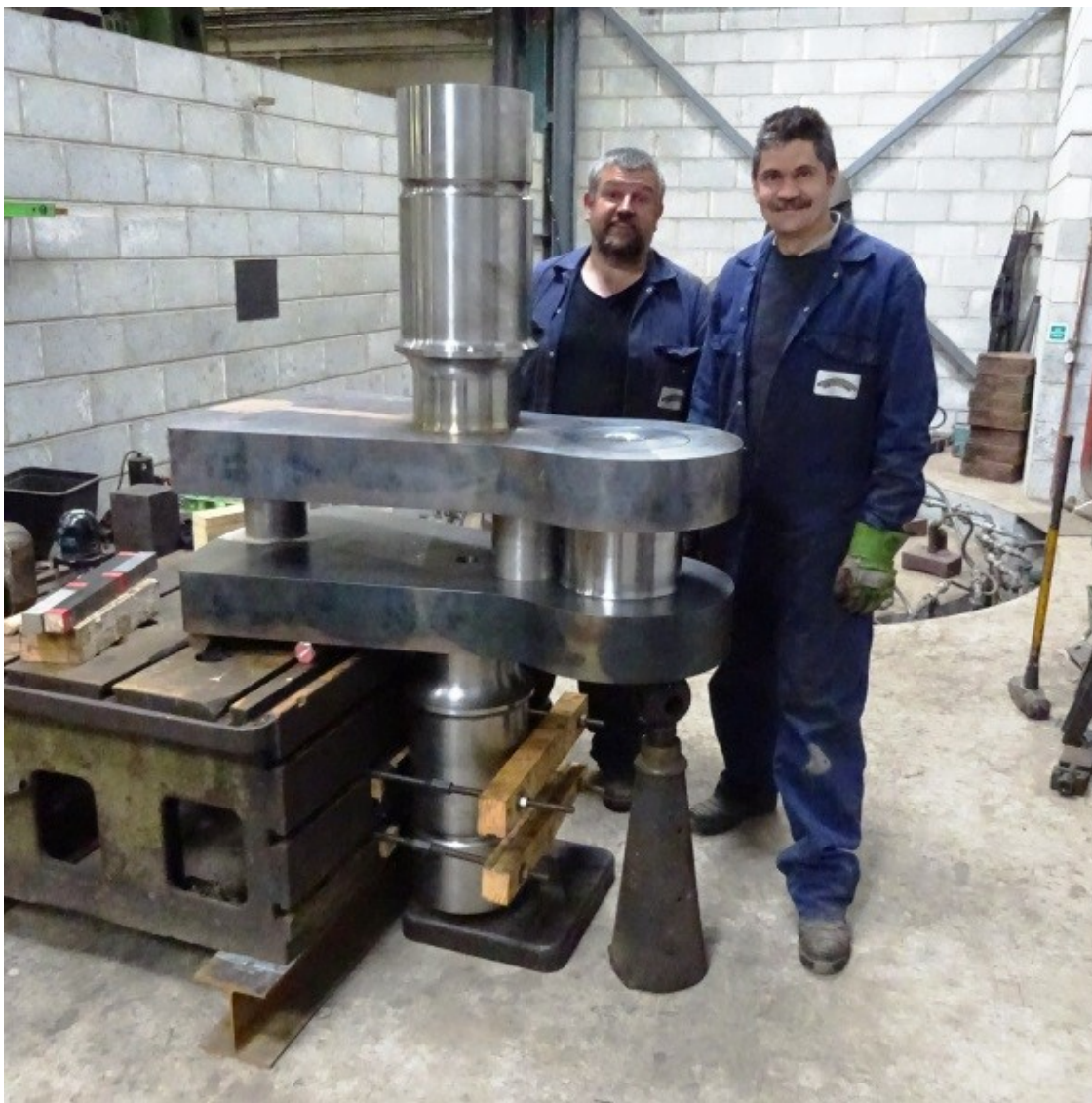
Rob Le Chevalier with the assembled crank axle at SDE - David Elliott
