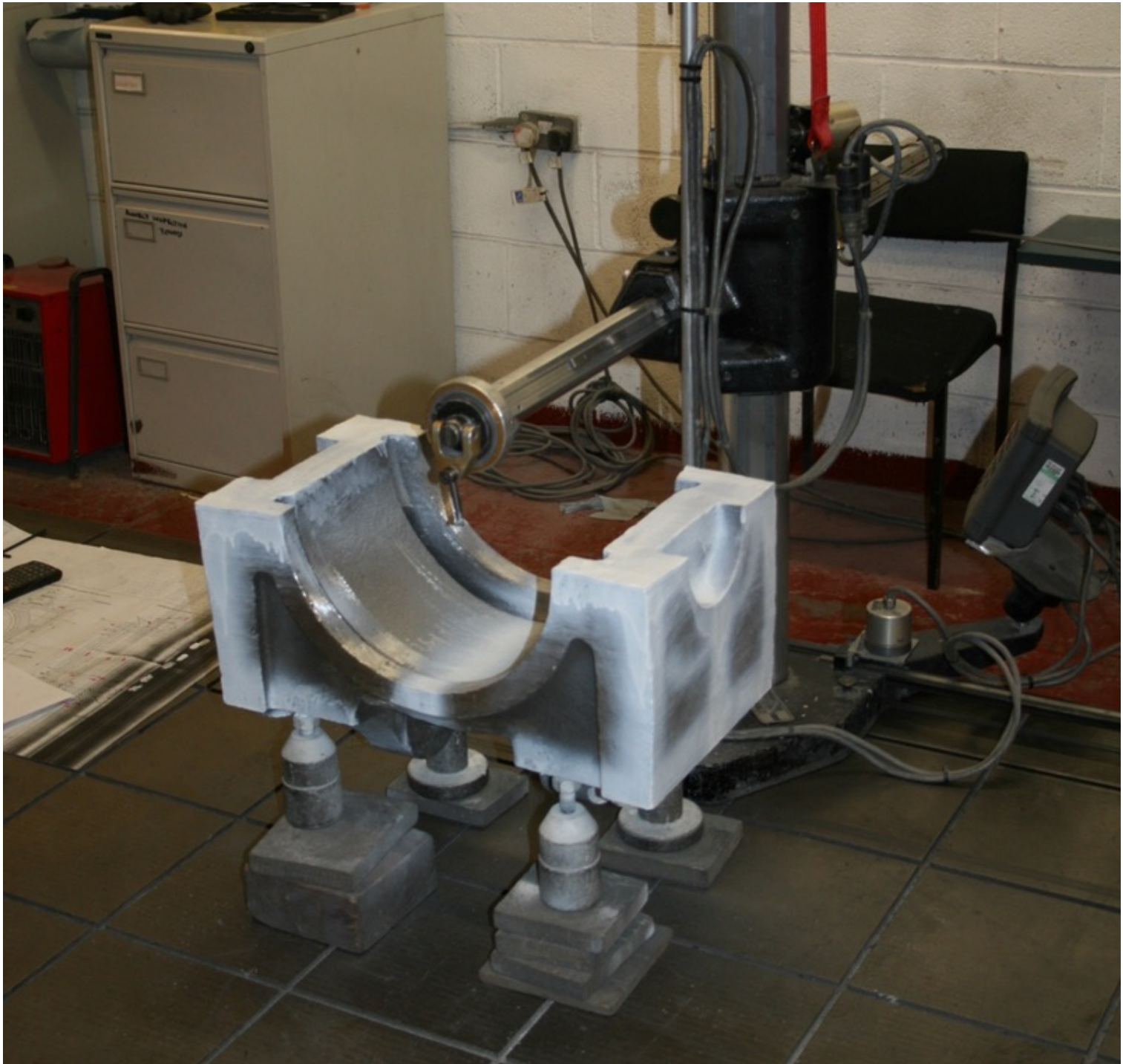
A coupled axlebox bottom casting on the measuring table at Cooks - David Elliott
