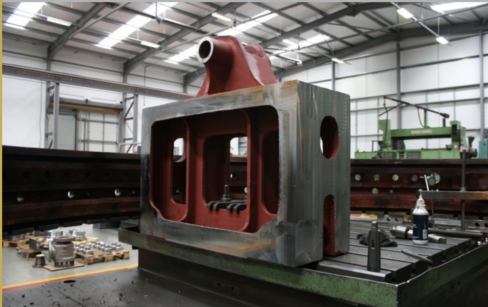
The drag box being machined at Multi-Tech - David Elliott
